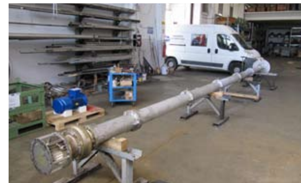
Intermediate pumps during assembly at the workshop
