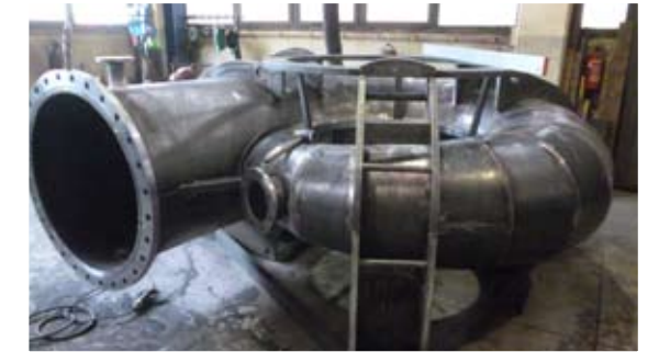
Welded monolithic structures for kaplan - francis - pelton hydraulic turbines Various amounts
