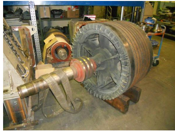
↓ C.G.E. 500 CV - 368 rpm - 3000 Volt - 50 Hz Cartoccio pumping plant for reclamation
