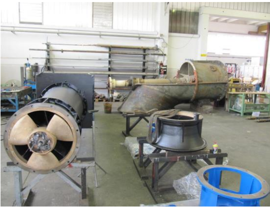
Repair of electric-pump Pellizzari type FIER 10.000 - Crevenzosa pumping plant
