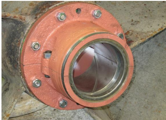
Cartoccio pumping plant - impeller - bearings in white metal - shaft protective bearings
