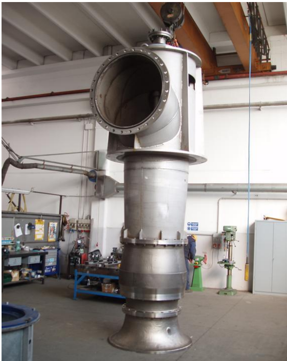
Mixed-flow pump interchangeable with the existing sited in a Petrochemical plant.
