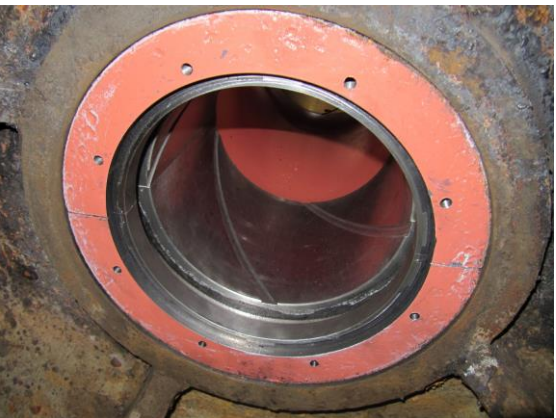
Cartoccio pumping plant - impeller - bearings in white metal - shaft protective bearings
