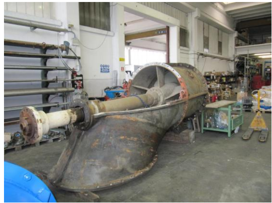
Repair of electric-pump Pellizzari type FIER 10.000 - Crevenzosa pumping plant
