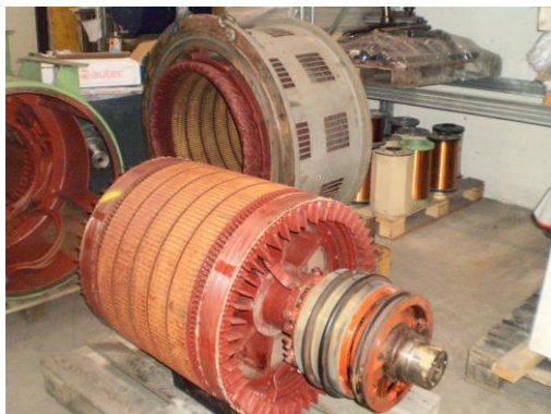
Overhaul of some electrical motors: with winded or short-circuited rotors.
