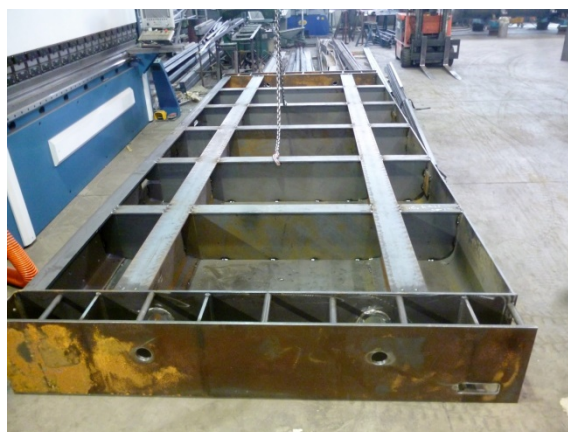
No. 1 Sluice gate for turbine protection 5,8 x 5,3 m, in carbon steel S355JR, hydraulic control
