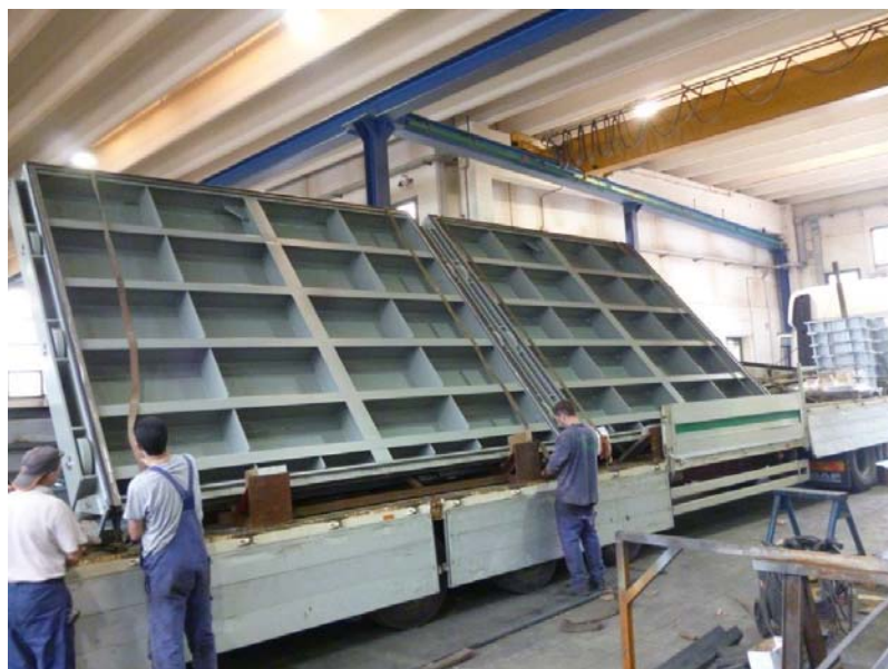
No. 6 Sluice gates, set on intake building 4,0 x 3,5 m, in carbon steel S355JR, hydraulic control
