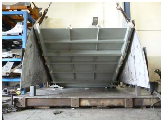
No. 1 Flap gate 2,40 x 1,90 m, in carbon steel S355JR, hydraulic control
