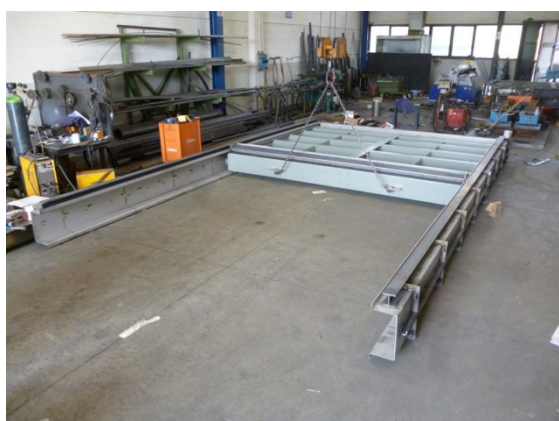
No. 1 Sluice gate for turbine protection 5,8 x 5,3 m, in carbon steel S355JR, hydraulic control
