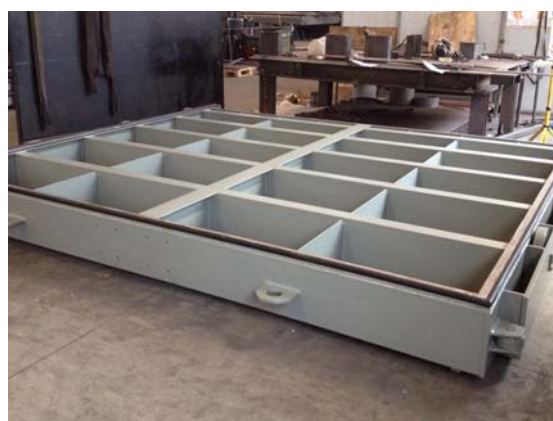
No. 1 Sluice gate for turbine protection 5,8 x 5,3 m, in carbon steel S355JR, hydraulic control
