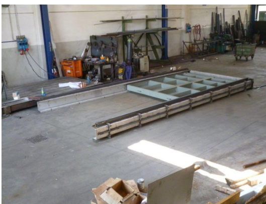
No. 1 Sluice gate for clean the river basin from stone and sand 2,77 x 3,30 m, in carbon steel S355JR, hydraulic control
